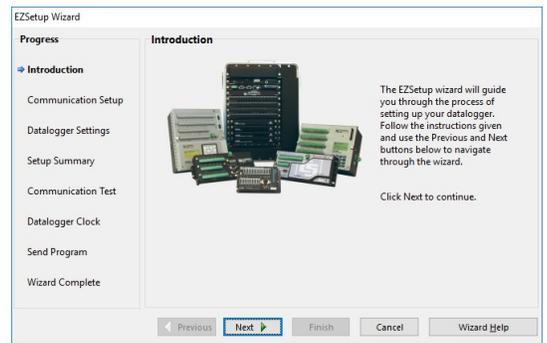
7. Configure the project folder path where data will be stored when it is collected from the logger. This can be done in **Data Files** page of the **EZSetup** wizard in LoggerNet's Setup application or from the **Collect Data** tab in PC200W's main window.
