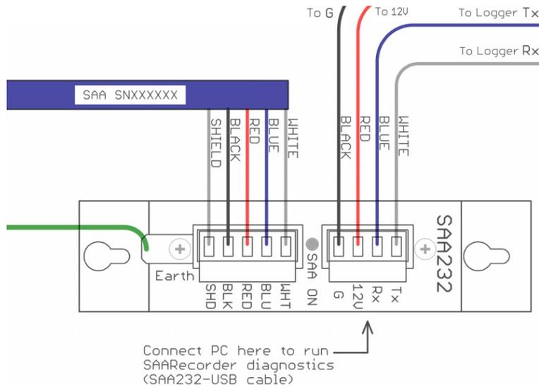
1. Physically connect the ShapeArray to an SAA232(-5). Connect the SAA232(-5) to a Campbell Scientific data logger.
