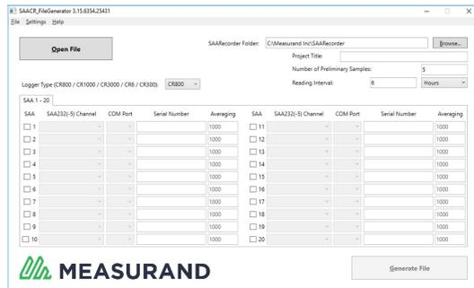
5. Start SAACR\_FileGenerator and configure the following fields: **Project Title**, **Number of Preliminary Samples**, **Reading Interval**, **Logger Type**, **232(-5) Channel**, **COM Port**, **Serial Number**, and **Averaging**. Click the **Generate File** button and provide a name for the program file.
